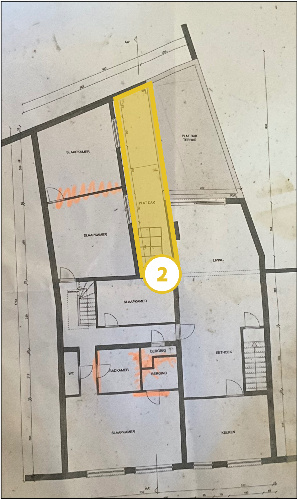
Legende van plan 1.5: Roofing plat dak
